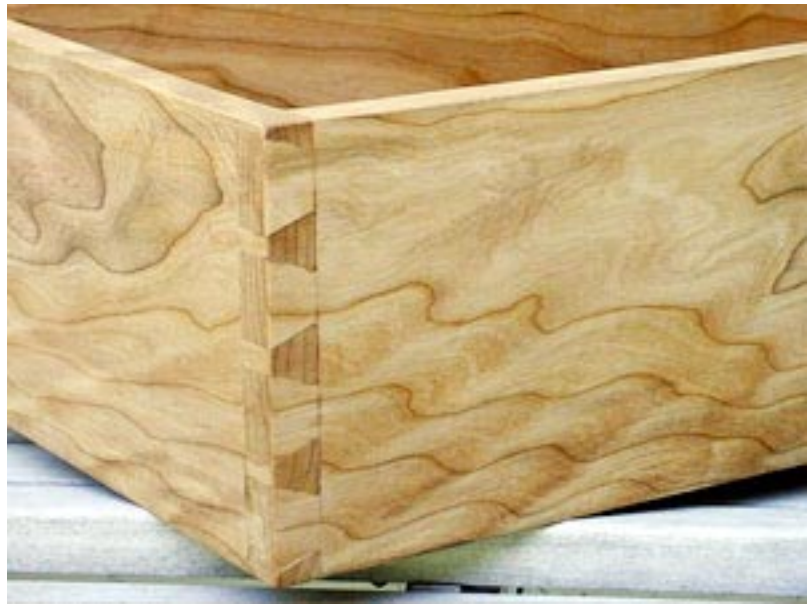
Attention To Detail ó Notice how the grain of this dovetailed box continues around the corner.
